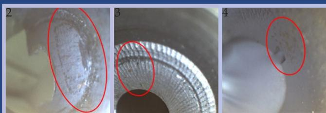
Figure 2: Debris within the large lumen of the device.
